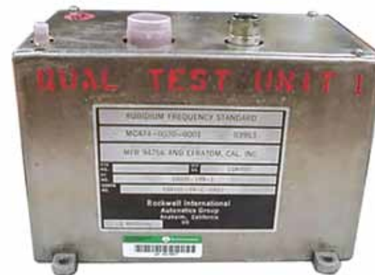
Qualification Model of the first GPS atomic clock, built by Rockwell International working directly with Efratom, a small German company.
