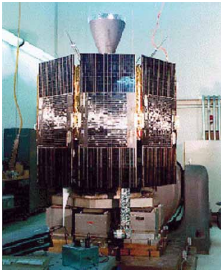
Timation NTS-1 carried two slightly modified commercial rubidium clocks. Unfortunately, attitude-stabilization problems induced temperature variations that masked any quantitative performance evaluation. The atomic clocks were not useful as prototypes for GPS.
