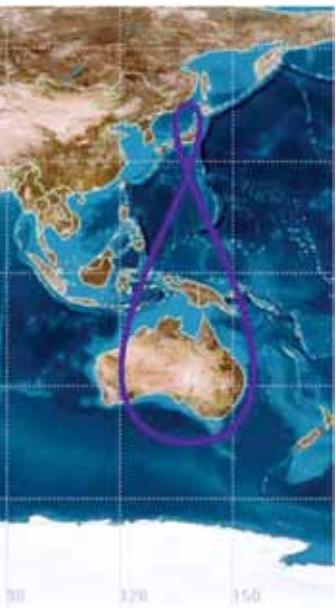
Figure 6. The Japanese QZSS has a similar constellation to an early proposal for GPS under 621
