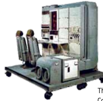
The Rockwell Collins Generalized Development Receiver (GDM). This advanced receiver achieved more than 100 dB of anti-jam in actual flight tests.
