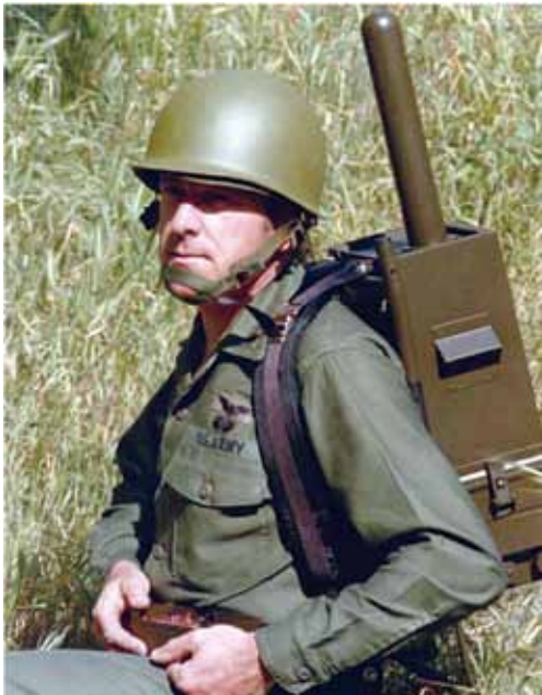
Early GPS manpack worn by JPO Army deputy Lt. Col. Paul Weber. This photo graced the cover of the first-ever GPS brochure.
